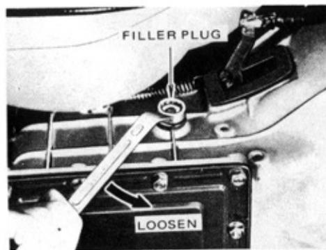
Remove the filler plug and feel inside the hole with your finger. The oil should come to the bottom edge of the hole. If the level is O.K., reinstall the plug and tighten it.
