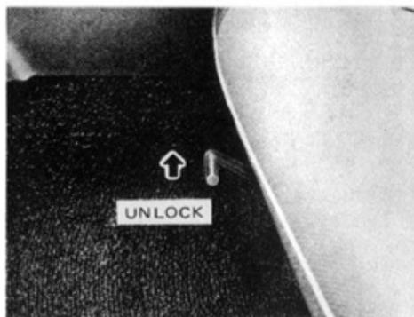
To move the seat forwards or backwards, pull the lock lever up. Then slide the seat to the desired position and release the lever.
