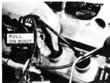
**1. Unfasten the spark plug cables by pulling on the boot, not on the cable itself.**
