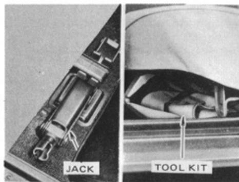
**STATION WAGON:** Get the jack out of the side panel on the left of the luggage compartment and the jack handle, together with the tool kit, from under the rear seat.
