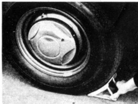
2. Block the wheel diagonally opposite the flat tyre to keep the car from rolling when it is jacked up.
