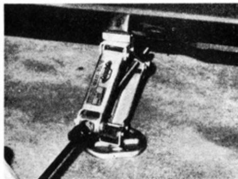
**6. Raise the car high enough for the spare tyre to be installed.**
