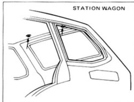
**On Station Wagon, the child restraint anchorages are in the rear roof by the back door hinge.**
