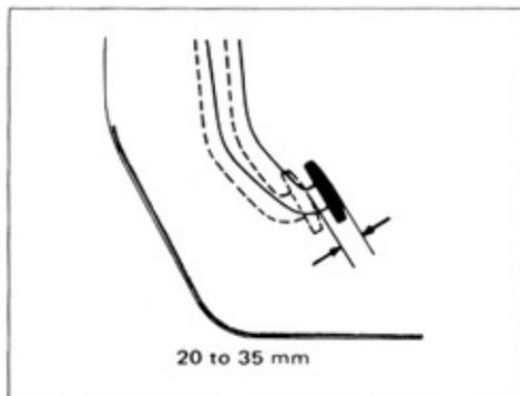
Press down lightly on the clutch pedal and measure the distance it moves freely before the clutch resistance is felt.
