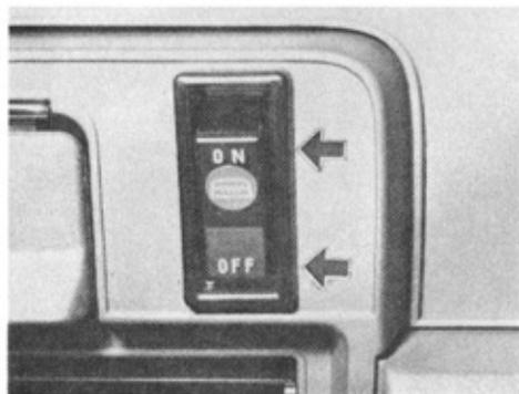
To turn on the electric defogger, push the switch with the engine running.
