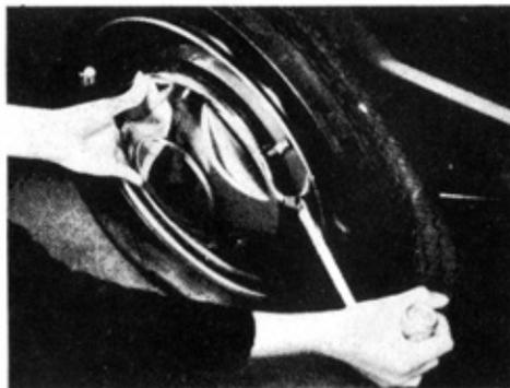
3. Using the end of the wheel nut wrench pry off the wheel cover, or the wheel hub ornament.
