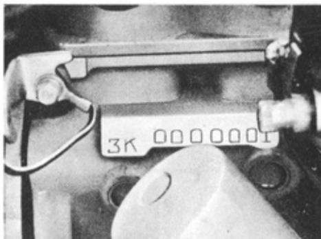
The engine number is stamped on the engine block as shown above.
