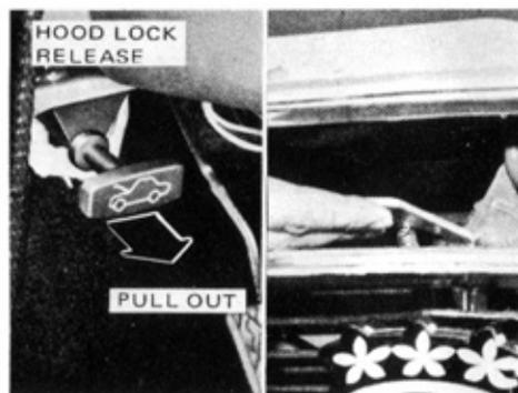
(1) Pull the hood lock release under the dash and the hood will spring up slightly. (2) In front of the car, press up the safety catch lever and lift the hood.
