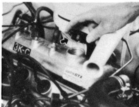
**1. Warm up the engine for a few minutes and remove the oil filler cap.**
