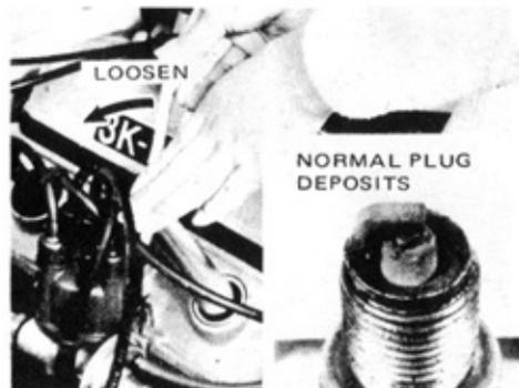
**2. Unscrew and remove the old spark plugs with their metal gaskets.**
