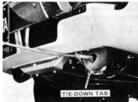
**For emergency towing, secure a cable or chain to the tie down tab under the front of the car.**
