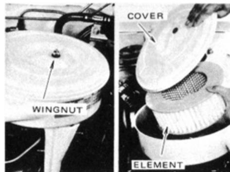
1. To inspect the element, unscrew the wingnut. Then remove the cover and lift out the element.
