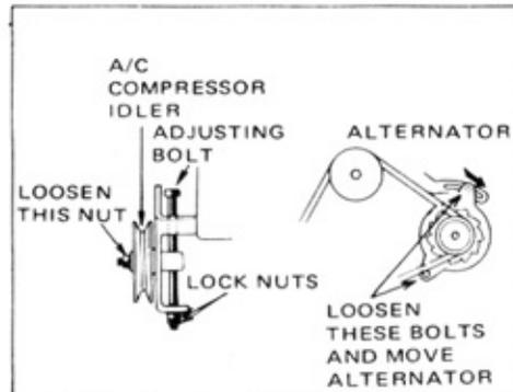
2. Use the screwdriver or bar to pry the moveable component outward until the desired belt tension is reached while holding the tension, tighten the adjusting bolts.
