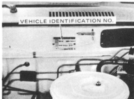
The Vehicle Identification Number (VIN) plate is installed in the engine compartment as shown above.
