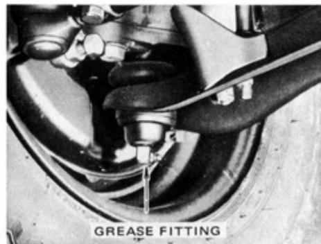
1. Remove the screw plug from the lower ball joint at the right and left side of the front suspension. Temporarily screw on a standard grease fitting.
