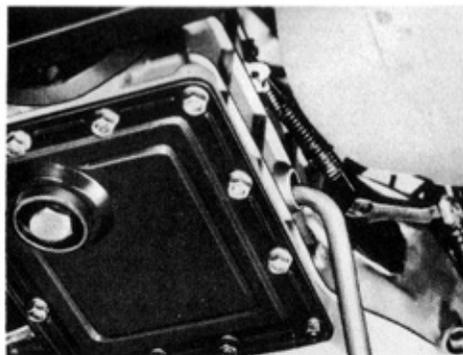
If the level is low, add SAE 80, API GL-4 gear oil until it begins to run out of the filler hole. Reinstall the plug securely.
