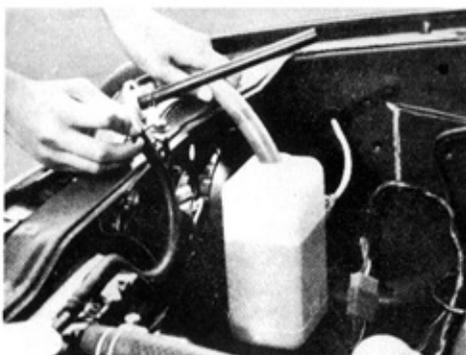
a. The cooling system must be treated with radiator coolant conditioner for corrosion protection. Insert the conditioner into the radiator (refer section 7 for amount to be inserted).
