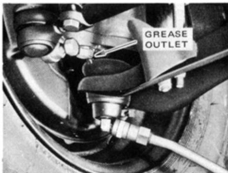
2. With the grease gun, pump lubricant (NLGI No. 1 or 2) into each fitting until it begins to flow from the grease outlet in the rubber dust boot. Remove the grease fitting and reinstall the screw plugs.
