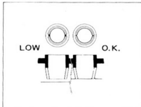
2. Depending on the type of battery installed in your car, check the electrolyte level as shown above. If the level is low, add distilled water.
