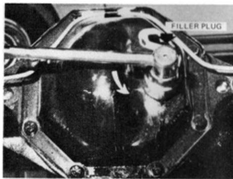
Remove the filler plug and feel inside the hole with your finger. If the oil comes to the bottom edge of the hole, the level is correct. Reinstall the plug.
