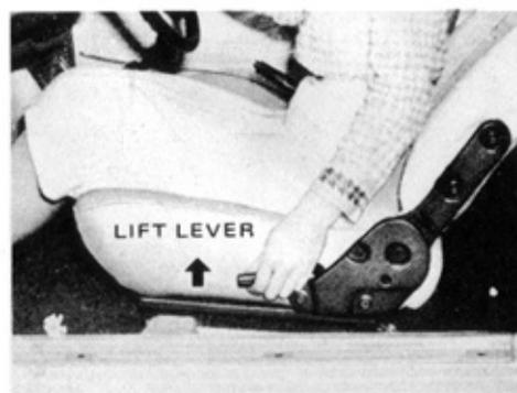
To change the seat back angle, lean forward and lift the lock lever. Then lean back to the desired angle and release the lever.
