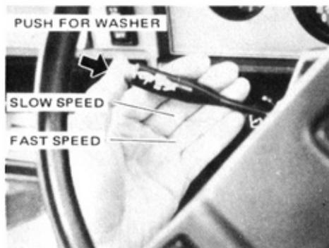
To turn the wipers on, pull the switch down. To make the washers squirt, push the button on the end.
