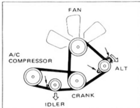
1. Loosen the adjusting bolts on each component, depending on the belt you wish to tighten.
