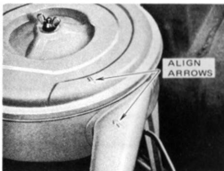
2. After installing an element, make sure the arrows on the cover and case are aligned. Then fasten the wingnut.
