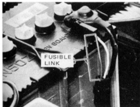
If the headlights or other electrical components do not work and the fuses are O.K., check the fusible link. If the link is melted, it must be replaced.
