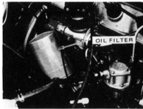
**3. Remove the old oil filter and install a new one, hand tight.**
