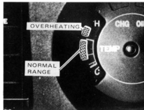
If the needle points to the red zone or higher, stop your car and allow the engine to cool.
