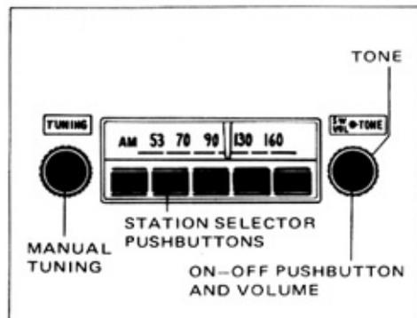
**Push the ON-OFF switch to turn the radio on. Another push will turn it off.**
