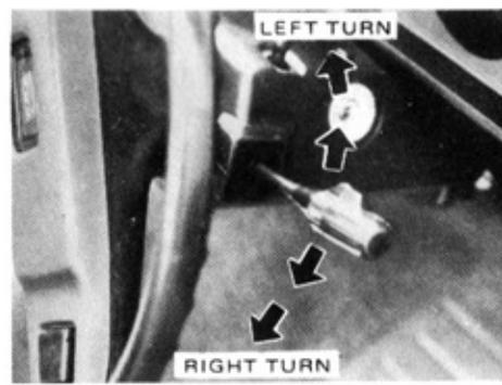
To turn the lights on, twist the knob on the end of the switch.
