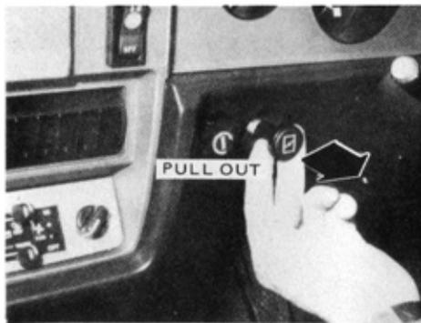
If the engine has not been running for several hours and the engine temperature gauge registers cold, pull the choke button half way out (refer section 2).
