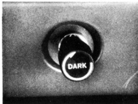
Turn the knob clockwise to dim the instrument panel lights.
