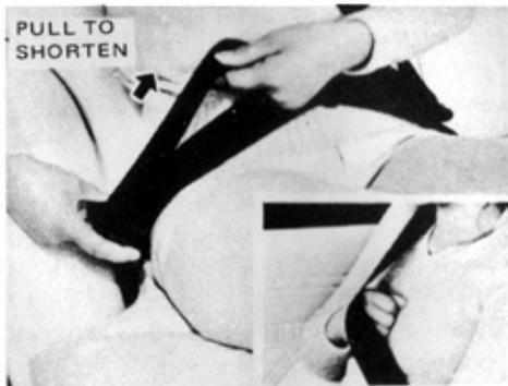
**3-point Type:** Adjust the length of the lap and shoulder belt.
