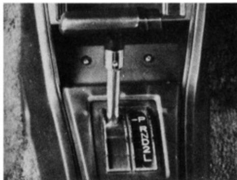
1. Check the fluid level only when the transmission is hot (normal operating temperature). With the engine idling, shift into every gear from PARK to LOW and return to PARK.
