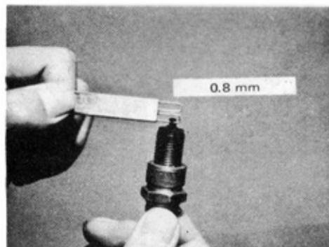
3. Set the gap on the new plugs to the correct clearance, and install them. Reconnect the spark plug cables in the correct order.
