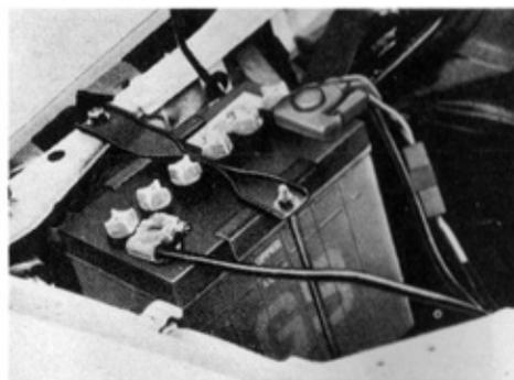
1. Check the battery for corroded or loose connections, cracks, or loose hold-down clamps.
