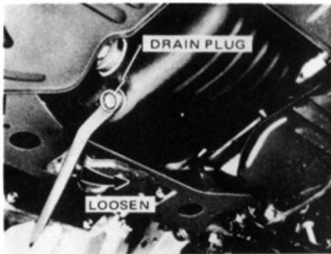
**2. Drain the oil and reinstall the drain plug.**
