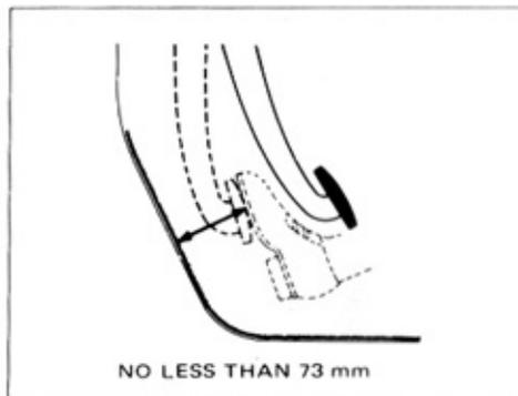
With the engine stopped, have someone press the brake pedal several times and then press hard on it. The distance from the floor to the top of the pedal should be no less than the above limit.
