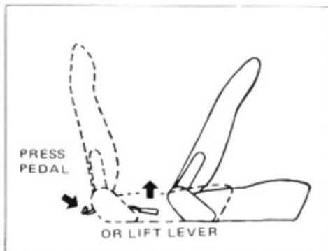
Lift the seat back lever or press the release pedal — the passenger's seat will automatically tilt forward.
