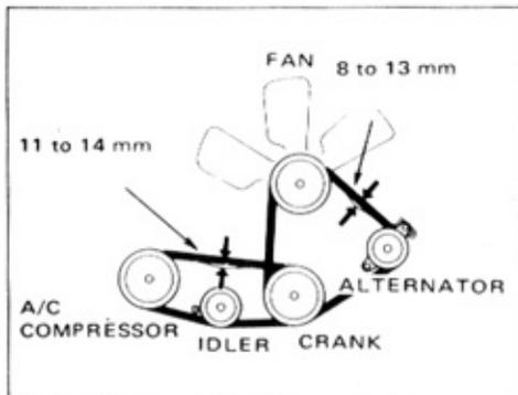
Visually inspect the condition of the belts. Check their tension by applying thumb pressure midway between the pulleys.
