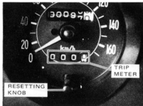
To set the trip meter, press the knob in and release it (option).
