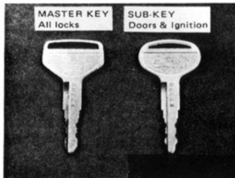
The master key works in every lock. The sub-key will work only in the ignition and doors.
