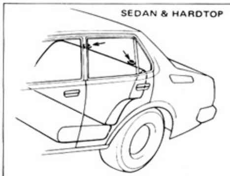
**On Sedan and Hardtop, take off a plug from the rear package tray and install a child restraint system with the anchor bolt.**
