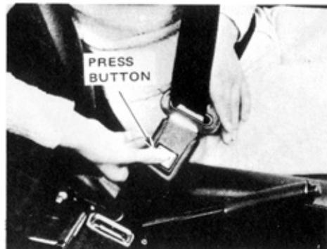
To release a belt, press the buckle-release button and allow the belt to retract.
