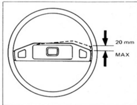
With the car stopped and the front wheels pointed straight ahead, rock the steering wheel gently back and forth.
