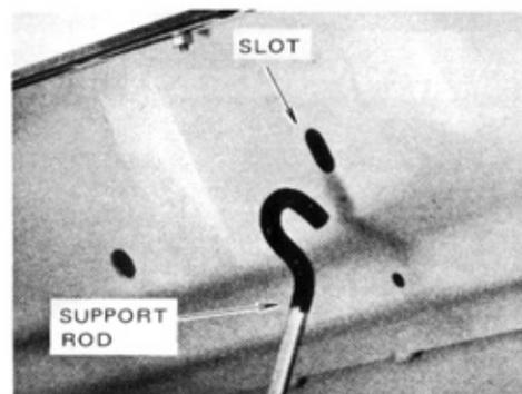
(3) After lifting the hood up, hold it open by raising the support rod into place.
