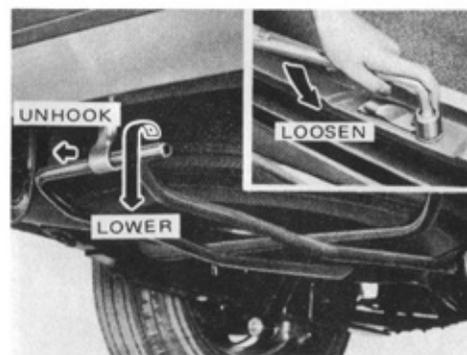
**STATION WAGON:** Loosen the spare tyre clamp bolt, pull the clamp away from the tyre holder, and lower the tyre.
