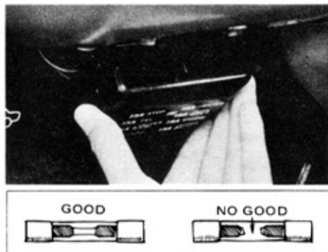
If any light or electrical component doesn't work, check to see whether the fuse has blown.
