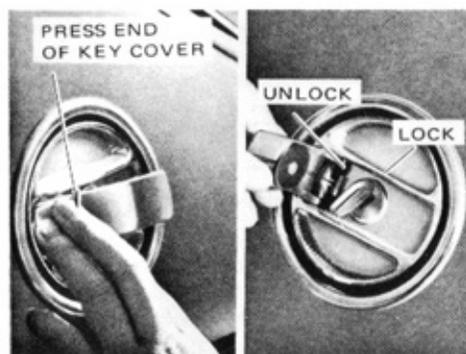
To refuel, unlock the tank inlet with your key, turn the cap counterclockwise, and lift it off.
