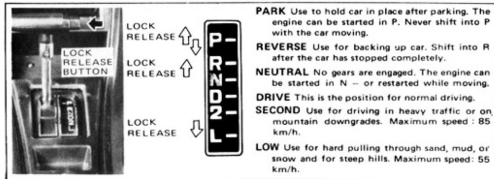
**PARK** Use to hold car in place after parking. The engine can be started in P. Never shift into P with the car moving.
